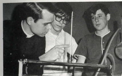
Brother James Reisz, physics teacher, helps his students at Boysville to determine the coefficient of linear expansion of a metal rod.
