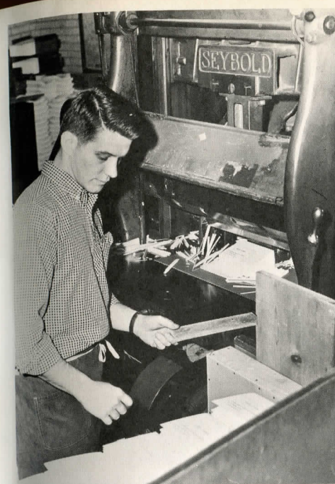
Seybold gives a help to Brother Richard Stull in trimming pamphlets on a three-knife trimmer.
